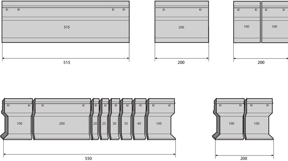
**Lunghezza e frazionature standard con Safety Click - Standard length and sectioning with Safety Click**
